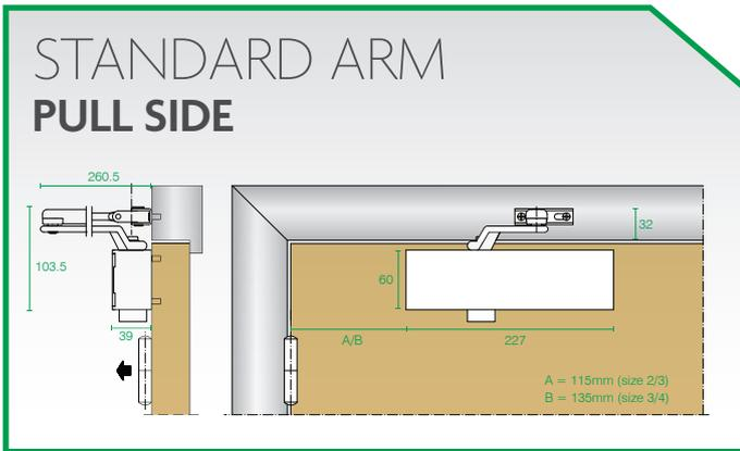
Provided the site conditions allow, an opening angle of 180 degrees is possible with this installation. Please note that using measurements A or B will provide different spring strengths.
