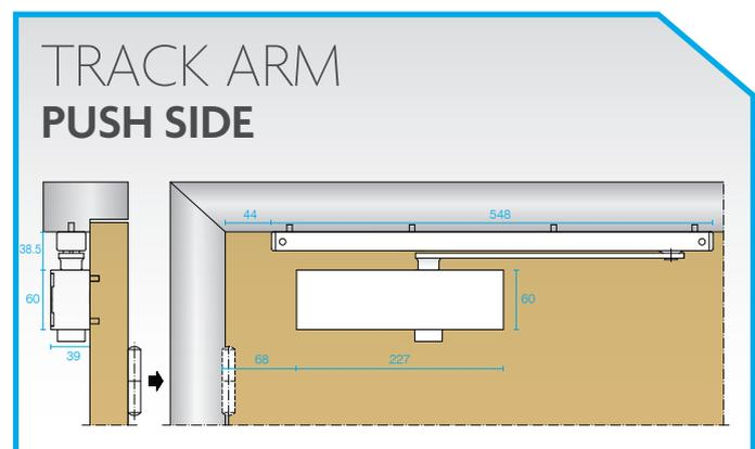
Provided the site conditions allow, an opening angle of 160 degrees is possible with this installation. Please note that using this installation a size 3 spring strength is achieved.
