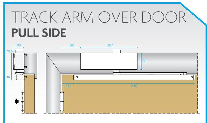
Provided the site conditions allow, an opening angle of 180 degrees is possible with this installation. Please note that using this installation a size 3 spring strength is achieved.
